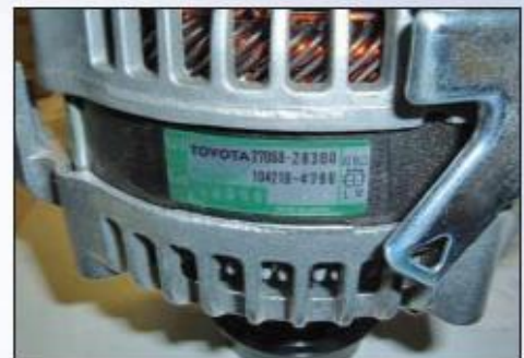
The photo's depict the RAV4 unit having a terminal callout IG-RLO-L-M. Inside you may find a regulator marked GC2M 3020; (this equates to OE Denso regulator number 126600-3020).
